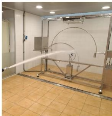
IPX6 POST TEST OBSERVATION: NO WATER INGRESSION OBSERVED INSIDE THE ENCLOSURE
